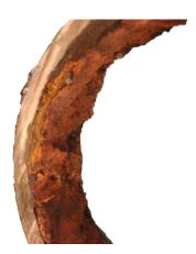
The effected pipe was placed in a 40% solution of TerraCleanse - ADH with water and left to soak for 6 hours.
